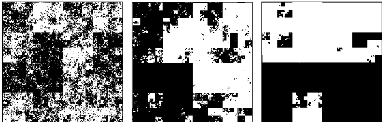
Figure 6. Curd-like fractals generated via a Haar wavelet synthesis. Hurst exponents are 0.0, 0.5, and 1.0 from left to right.
